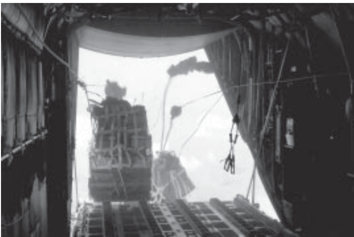
Joint Precision Air Drop System bundles fall out of the back of a C-130 Hercules Aug. 25. The drop was made from almost 10,000 feet above sea level and was calculated using up-to-the-minute wind data relayed from two small dropsondes deployed 20 minutes earlier. The dropsondes calculate wind speed and relay the information back to the aircraft, helping to calculate the correct drop point. (U.S. Air Force photo/Senior Airman Brian Ferguson)
